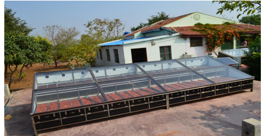
SOLAR CABINET DRYER - SDM-400 MODEL
